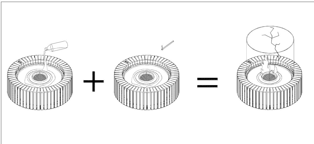
**EN** Igniting the spilled fuel is extremely dangerous and will cause the glass tube to crack. **Glass tube is not covered by the warranty.**
